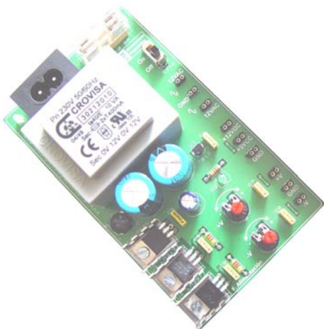
Figure 2-1. The power supply
